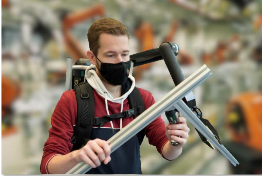
Trimanual assembling using a supernumerary robotic arm as will be developed by ISIR Sorbonne within the NIMA project.
